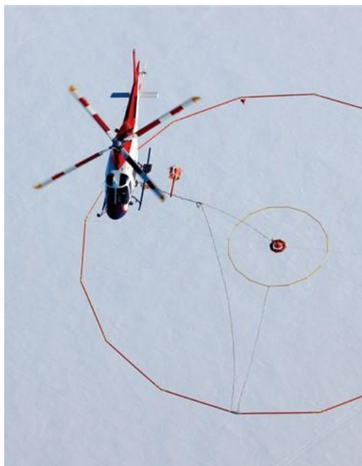
Geotech Ltd. VTEM helicopter time-domain EM system (courtesy Geotech Ltd.)
